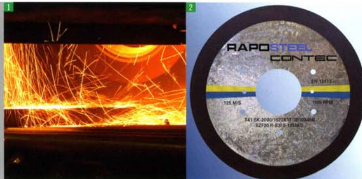
1. Large diameter cut-off wheel in action 2. Large diameter cut-off wheel with recyclable core
